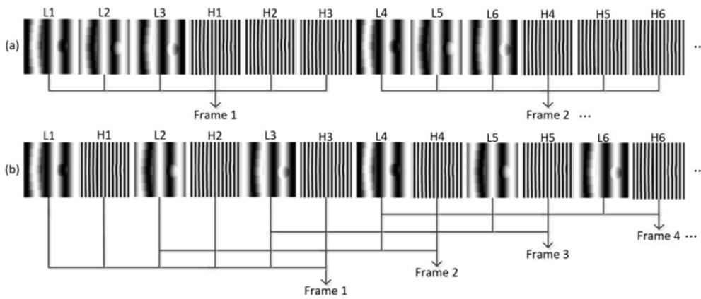
Fig. 3. The strategy of the fringe pattern projection. (a) The frame rate of the traditional PSP with dual-frequency phase unwrapping method; (b) The frame rate of the proposed strategy with dual-frequency phase unwrapping method. (For interpretation of the references to color in this figure legend, the reader is referred to the web version of this article.)
