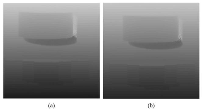
Fig. 6. The compensation of the phase map. (a) The unwrapped phase map of low frequency before compensation; (b) The unwrapped phase map of low frequency after compensation and position adjustment.
