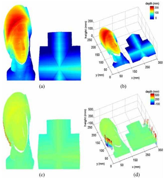
**Fig. 8.** The reconstructed results of the object with complex surface. (a) The reconstructed result with the proposed method; (b) The mesh display for Fig. 7(a); (c) The reconstructed result with the traditional method; (d) The mesh display for Fig. 7(c).
