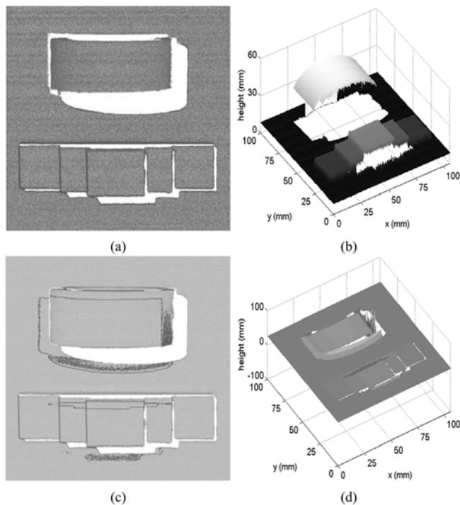
**Fig. 7.** The reconstructed result with the proposed method and traditional method. (a) The reconstructed result with the proposed method; (b) The mesh display for Fig. 7(a); (c) The reconstructed result with the traditional method; (d) The mesh display for Fig. 7(c).
