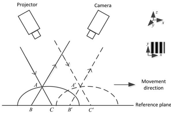
Fig. 2. The measurement system with moving object.
