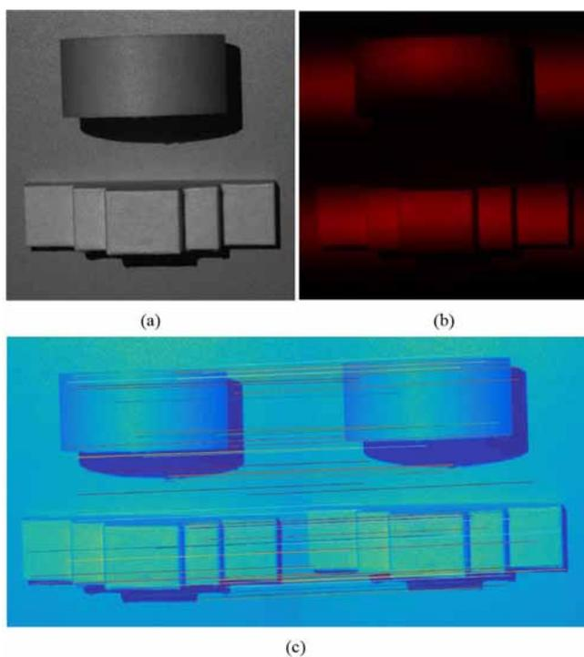
Fig. 4. Two isolated objects used in the experiment. (a) The two isolated objects used in the experiment; (b) The captured object image in red fringe pattern; (c) The movement tracking result with SURF algorithm. (For interpretation of the references to colour in this figure legend, the reader is referred to the web version of this article.)
