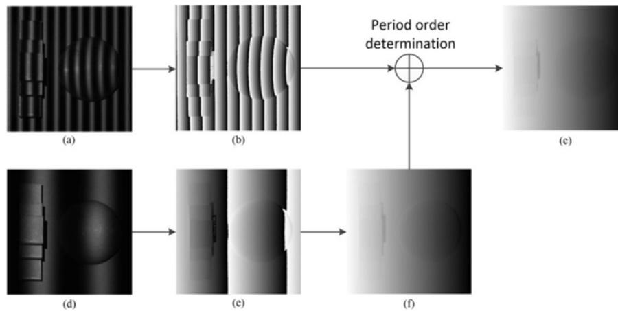
Fig. 1. The procedure of the dual-frequency phase unwrapping method. (a)–(c): the captured fringe pattern, the wrapped phase map and the unwrapped phase map of high frequency fringe pattern; (d)–(f): the captured fringe pattern, the wrapped phase map and the unwrapped phase map of low frequency fringe pattern.
