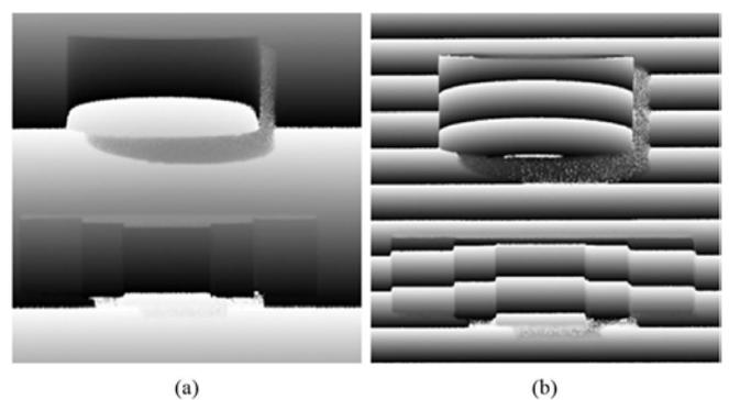
Fig. 5. The wrapped phase maps of the low frequency and high frequency. (a) The wrapped phase map of low frequency; (b) The wrapped phase map of high frequency.
